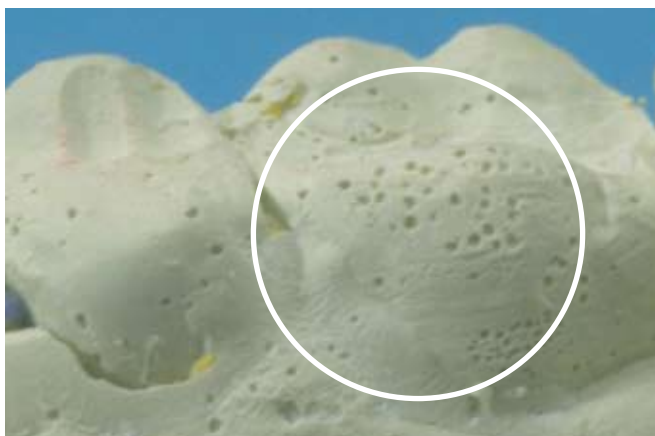
Stone Model with Hydrogen Evolution Voids
